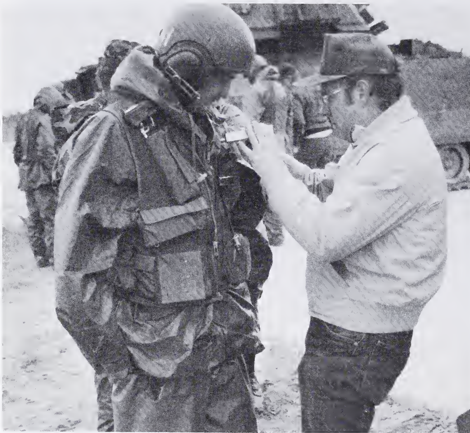
A Bradley Fighting Vehicle crewman being equipped with breathing-zone sampling equipment for the capture of atmospheric samples of weapons combustion products in a test conducted by the U.S. Army Biomedical Research and Development Laboratory.
